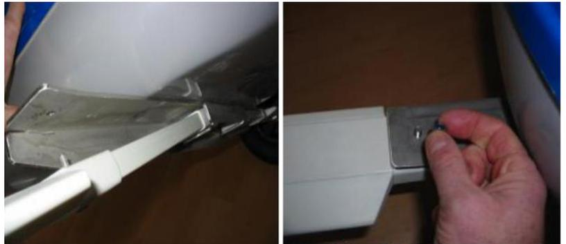
*Mount the axles under the support by inserting the rubber tip inside the rectangle hole and thread the hole at the extremity of the support with the screw of 6mm which is fixed on the axles. Next step is to tighten the nut to secure the fixation.*
