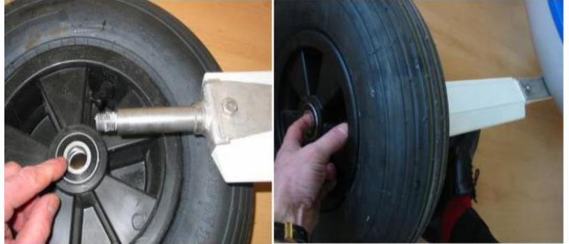
*Mount the wheels on the axles. Small or large back wheels: Insert the wheel in the spindle by aligning the spacer tube with your index finger. Mount the axles support to the body with 2 nuts of 13mm.*
